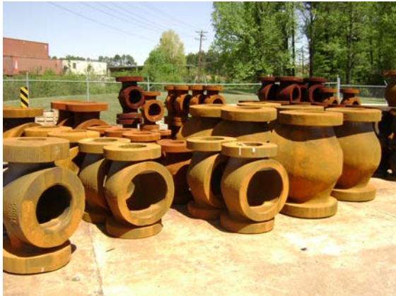
Bare castings stored outside; heavy rust
