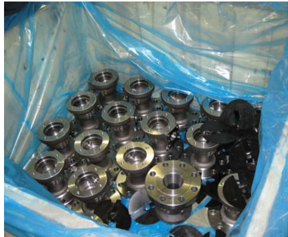
New method with Defender bag and ARMOR WRAP® VCI Paper interleave. No oil used.
