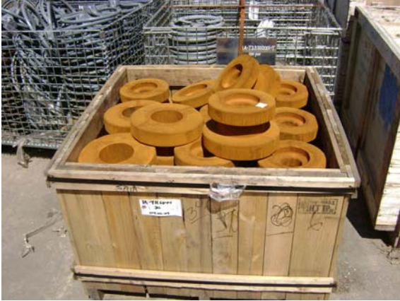
Bare castings outside with heavy rust
